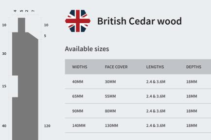
Illustration shows TG&V cladding profile in British Cedar wood at 140mm width. Not to actual scale.
